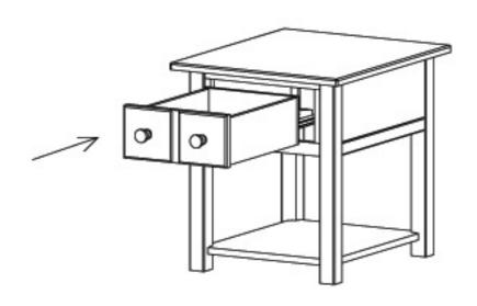
DO NOT TIGHTEN SCREWS UNTIL COMPLETELY ASSEMBLED
