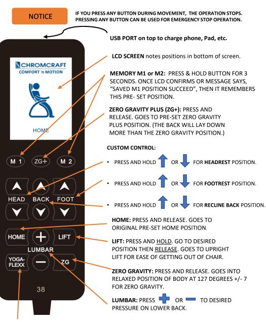
**YOGA FLEXX:** PRESS & RELEASE 1 time- to go for 5 MINUTES, PRESS 2 times for 10 MINUTES, PRESS 3 times for 15 MINUTES, PRESS the 4<sup>TH</sup> TIME- to **STOP**. *(This is a CYCLED INTERVAL MOTION for spinal stress-reducing relaxation.)*
